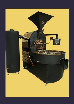
ROS15 coffee roaster has been designed for optimal and high efficiency heat transfer and distribution. Our development on coffee roasting brings the unique drum design which has homogeneous, constant and stable bean roasting at each batch.
